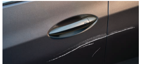
1 dent or 2 scratches (more than 4") per panel
