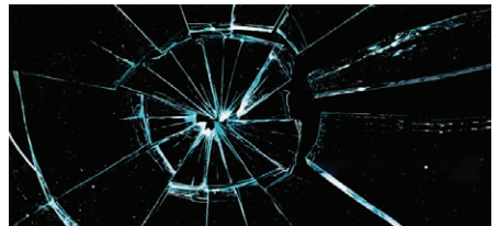
Cracked glass more than 1/2" in diameter or spidered cracks
