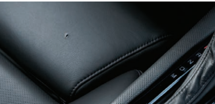
Upholstery holes equal to or less than 1/8"
