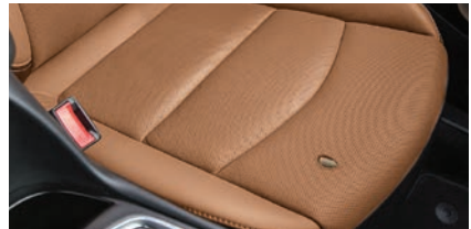
Upholstery holes more than 1/8"
