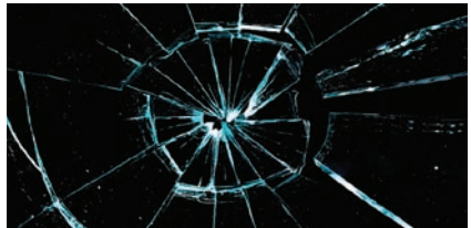
Cracked glass more than 1/2” in diameter or spidered cracks
